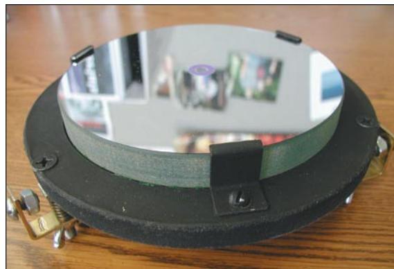
Fig. 5 Mirror with diameter 6 inches and depression 0.05 inches before installation in class-made telescope
